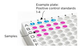
Seal the plate carefully and spin it briefly in a plate centrifuge to ensure that all the reagents are at the bottom of the well. Load the plate into the qPCR instrument.
